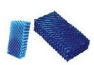
made up of virgin PVC which are mounted on Pultruded FRP structural member. Available in 12, 19 and 27 flutesize as per requirement. The fills shall withstand a maximum inlet water temperature of 55°C.
